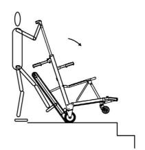
When all the wheels reach the staircase landing, release the UP button, grip the handle and slowly lean forward to make four wheels stand on the ground.
