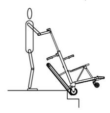
After the belts pass the first stair step, adjust STAIRCLIMBER slowly to let the belts cover two/ three steps along the staircase angle,.
