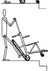
When the front wheels reach the staircase edge, tilt the chair backward until the track belts on the floor as shown, then press the DOWN button.
