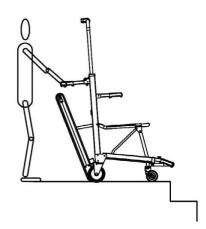
Grip the rear lifting handles push STAIRCLIMBER to next location.
