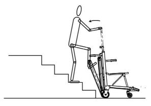
Adjust the distance (30- 40cm) between the rear castors and the staircase slowly tilt the handle back until the track belt lean on the stair steps as shown.
