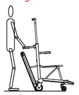
Deploy STAIRCLIMBER as shown; make sure that the battery switch is on, adjust the telescopic frame to suitable height.
