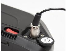
Connect the DC power adapter at to the battery charging port as (connect the other end as to wall socket) to charge, and make sure the battery is fully charged before using the stair climber. When the indicator lamp as on the battery turns green from red, it means that the battery is fully charged.
