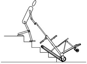
Press POWER button to start lifting the chair, meanwhile press the gripping frame a little to make the track belts cling to stair steps.
