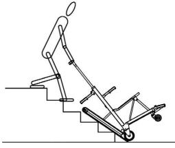
When the track belts reach the floor at the bottom of the stairs release the DOWN button, then slowly tilt the chair forward until the four wheels stand on the floor.
