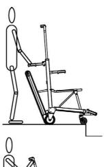
Push STAIRCLIMBER to staircase, adjust the chair and make the track belts at the middle of the staircase.
