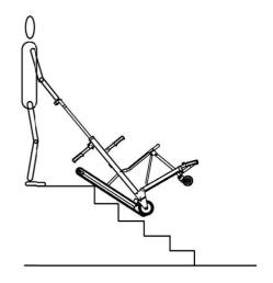
If need to pause or stop, release DOWN button. Note: when the track belts cover one or two steps, press the handle downwards a little to avoid STAIRCLIMBER leaning forward.
