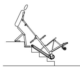
If need to pause or stop, release UP button. Note: when the track belts lie on one or two stair steps, make sure to press the frame downwards to avoid STAIRCLIMBER leaning forward.
