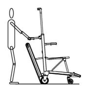
Deploy STAIRCLIMBER as shown, be sure the battery is switched on, adjust the telescopic gripping frame to suitable height.
